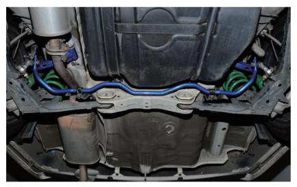
Torque for bolts 螺絲鎖緊扭力: M8-60Nm M10-80Nm
